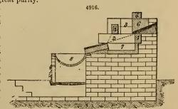
diagonally across it. The space between the under surface of the work-stone and the brick or stone bed is generally fitted up with fire-clay, or with a mixture of slime-ore and bone ashes tempered with water.
